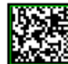
Quiet zone violation
