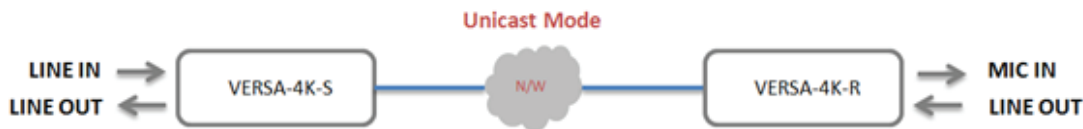
Fig 15: Bidirectional Audio Pass-Through
