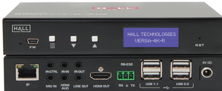
Fig 3: VERSA-4K-R Front and Rear panel
