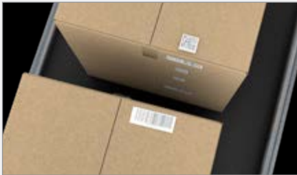
Short gaps between packages make uniform lighting difficult
