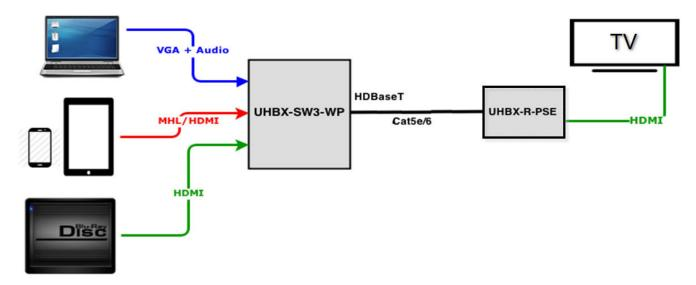
The above diagram shows the three inputs on the UHBX-SW3 (one VGA and two HDMI), as well as the Receiver (UHBX-R-PSE) to which the TV is connected.
