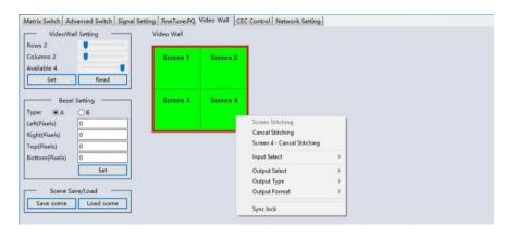
Once connected, G44H will load the settings used from last time. The default setting for the new unit out of package is 2x2 video wall with input 1 across the 4 screens. All outputs are set at resolution of 1920 x 1080@60.
