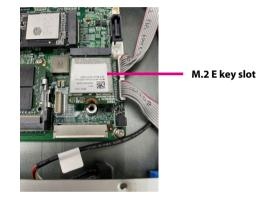
3. Push the module down and secure it with the screw that was removed from step 1.
