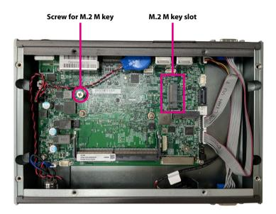
2. Insert the M.2 module into the M.2 slot at a 45-degree angle until the gold-plated connector on the edge of the module completely disappears into the slot.
