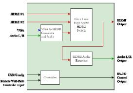
Figure 1 - Internal Block Diagram
