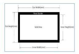
Users can set up the bezel correction for the video walls here to compensate the frame of the screens to make the whole video wall look like one large screen without any distortion. Users can use pixels of the screen frame width to set up the bezel correction here. The bezel compensation can be set either ON or OFF for comparison.
