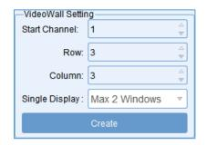
Users can set up the layout of the video wall in 'VideoWall Setting' by simply choosing the number of rows and columns in the video wall. Total screen amount is up to 8/12/16 for SWMicro video wall controllers depending upon the model type.
