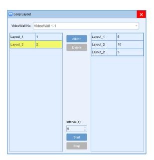
Users can save the video wall layouts and recall them later via the 'Layout' menu on the left of the software. Users can save up to 32 pre-set layouts.
