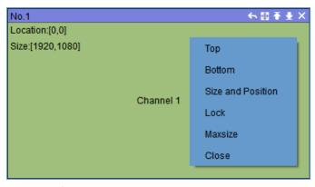
Right click on the video wall, users can use the tools in '**Dropdown menu**' to set up each window individually. Some of these functions can be accessed using the tool bar on the right-top of each window.
