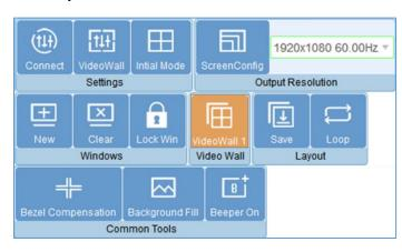
Once connected, SWMicro will load the settings used from last time. The default setting for the new unit out of package is 2x4/3x4/4x4 video wall with input 1 across the screens depending upon the model type. All outputs are set at resolution of 1920x1080@60hz. The function of each tab on the main window for setting up a video wall will be:
