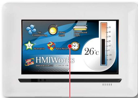
7" TFT LCD with Touch Panel
