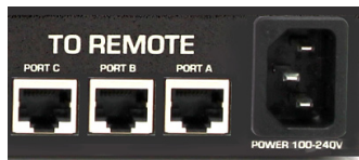
Close-up of Sender UTP Connections
