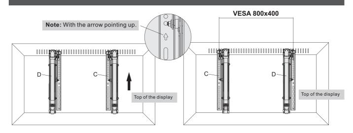
For VESA 800x400, the positions of "D" and "C" are exchanged.
