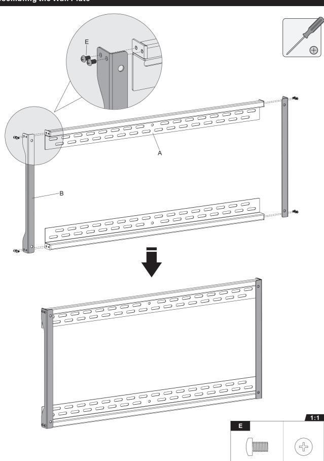
Attach the connecting plates to the wall plates using the appropriate screws.
